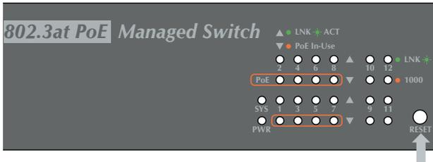
Figure 10-2: GS-4210-8P2T2S Reset Button
