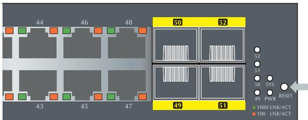
**Figure 10-5:** GS-4210-48T4S Reset Button
